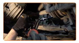
Remove the hydraulic transmission jack.
