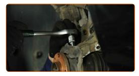
Release the fastener connecting the ball joint to the steering knuckle. Use a flat metal-working chisel. Use a hammer.
