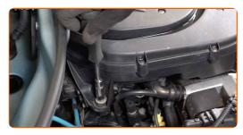
Remove the air filter housing retaining spring.
