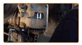
Connect the brake pad wear sensor plug.
