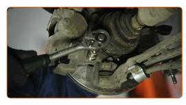
Connect the brake hose fastener to the shock absorber strut.
