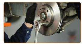
39.1 Install the brake caliper together with its bracket.
