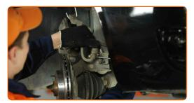
Unscrew the brake disc fastening. Use a drive socket #12. Use a ratchet wrench.
