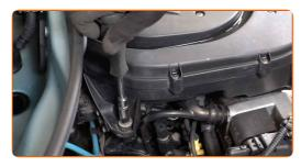
Remove the air filter housing retaining spring.
