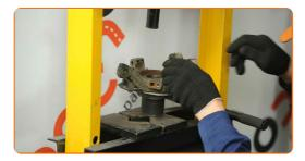
Press the new bearing in the steering knuckle.
