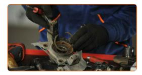
Press out the wheel hub bearing.
