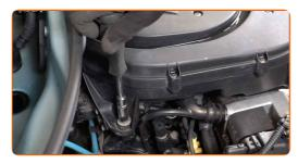
Remove the air filter housing retaining spring.
