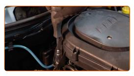
Install the air filter housing retaining spring.
