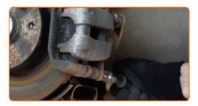
Remove the brake caliper. Use a crowbar.
