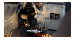
11 Remove the brake caliper.
