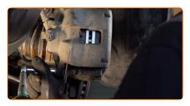
Connect the brake pad wear sensor plug.
