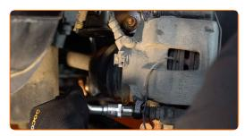
11 Remove the brake caliper.
