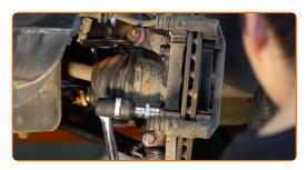
Remove the caliper bracket.
