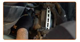
Tighten the brake caliper bracket. Use a drive socket #19. Use a torque wrench. Tighten it to 110 Nm torque.
