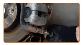
Remove the brake caliper. Use a crowbar.
