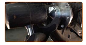
Treat the hub where it contacts the brake disk. Use copper grease.
