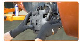
Install the brake caliper cotter pin. Use a pin punch. Use a hammer.
