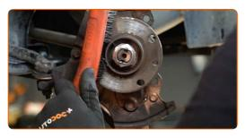
Clean the brake disk surface. Use all-purpose cleaning spray.
