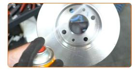
21 Install the brake disc.
