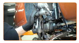
Tighten the brake caliper bracket. Use a drive socket #18. Use a torque wrench. Tighten it to 55 Nm torque.
