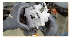
12 Remove the brake pads.
