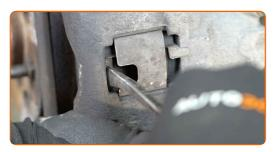
Remove the lock pin retainer clip. Use round-nose pliers.
