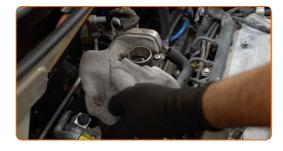
17 Reinstall the air filter housing.
