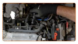
Screw new spark plugs and tighten them. Use the spark plug socket #16. Use a torque wrench. Tighten it to 25 nm torque.
