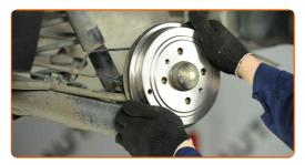
Tigten the brake drum fasteners. Use a drive socket #12. Use a torque wrench. Tighten it to 15 Nm torque.
