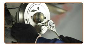
Remove the brake drum.
