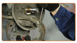
Clean the brake drum. Use a brake cleaner.
