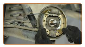
Reinstall the brake shoe hold-down cup.
