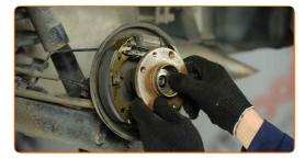
Tighten the hub. Use a drive socket #32. Use a torque wrench. Tighten it to 280 nm torque.
