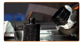
17 Remove the oil filter cover O-ring. Use a flat screwdriver.
