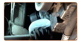
Unscrew the filter housing cap together with the old filter element.
