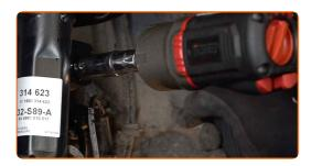
Unscrew and remove the wheel arch cover fasteners. Use a drive socket #10. Use a ratchet wrench. Use a Phillips screwdriver.
