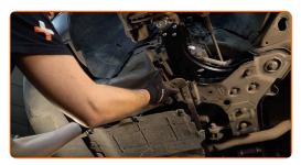
Install and tighten the wheel arch cover fasteners. Use a drive socket #10. Use a ratchet wrench. Use a Phillips screwdriver.
