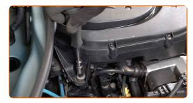
Remove the air filter housing retaining spring.
