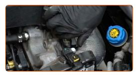
Tighten the oil filler cap.
