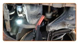
Unscrew the drain plug. Use HEX No.H12. Use a ratchet wrench.
