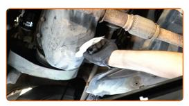
Screw in the new drainage plug and tighten it. Use HEX No.H12. Use a torque wrench. Tighten it to 22 Nm torque.
