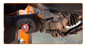
Remove the brake caliper.
