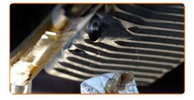
Screw in the new drainage plug and tighten it. Use a drive socket #13. Use a torque wrench. Tighten it to 28 Nm torque.
