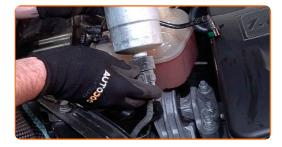
Attach the fuel pressure sensor connector.
