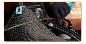
Screw in the fuel filter bleeder screw. Use a drive socket #12. Use a ratchet wrench.
