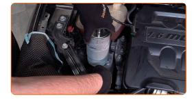
Detach the fuel pressure sensor connector.
