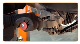
Remove the brake caliper.
