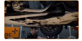
Clean the stabiliser link fasteners. Use a wire brush. Use WD-40 spray.
