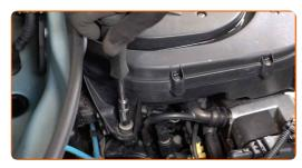
Remove the air filter housing retaining spring.
