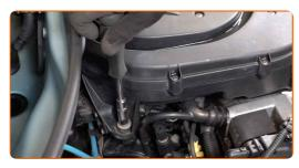
Remove the air filter housing retaining spring.
