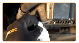
Screw in the new drainage plug and tighten it. Use a drive socket #17. Use a torque wrench. Tighten it to 22 Nm torque.
