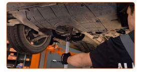
Remove the oil pan cover. Remove the hydraulic transmission jack.
