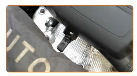
6 Remove the air filter housing.
