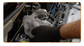
17 Reinstall the air filter housing.
