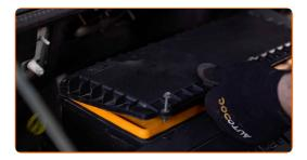
Screw in the fastening screws of the air filter cover. Use a drive socket #8. Use a ratchet wrench.
