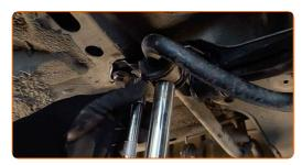
Remove the transmission jack from under the stabilizer bar.
