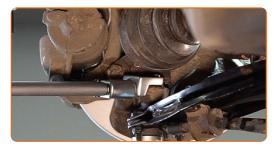
Remove the support from under the arm.
