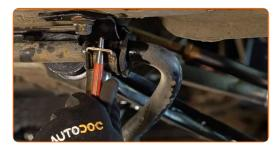
Screw in the fastener of the bracket that connects the stabilizer bar to the car body. Use a drive socket #13.
