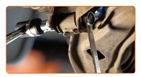
Unscrew the fastener of the bracket that connects the control arm to the car body. Use a drive socket #15.
