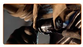
Connect the lower arm to the steering knuckle.
