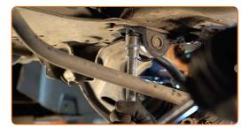
18 Remove the front fastener of the control arm.
