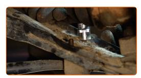
Disconnect the stabilizer bar from the control arm. Use a crowbar.
