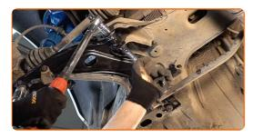
Tighten the ball joint fastener. Use a combination spanner #19. Use a torque wrench. Tighten it to 60 nm torque.
