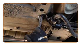
Tighten the fasteners that connect the stabilizer bar to the suspension control arm. Use a drive socket #13. Use a torque wrench. Tighten it to 28 nm torque.
