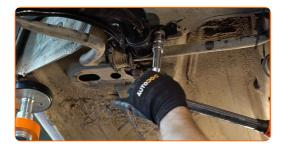
Tighten the fastener of the bracket that connects the control arm to the car body. Use a drive socket #15. Use a torque wrench. Tighten it to 50 nm torque.
