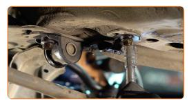
Unscrew the rear arm fastener. Use a drive socket #18. Use a tap wrench.
