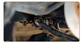
Unscrew the fastening bolts of the bracket that connects the stabilizer bar to the car body. Use a drive socket #13.
