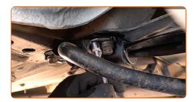
Tighten the rear fastener of the control arm. Use a drive socket #18. Use a torque wrench. Tighten it to 80 nm torque.
