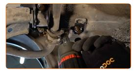
Unscrew the fastening bolts of the bracket that connects the stabilizer bar to the rear side of the control arm. Use a drive socket #18. Use a tap wrench.
