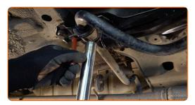
Align the fastener holes of the stabilizer link and the suspension control arm. Use a pin punch.
