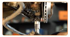
Screw the front arm fastener. Use a drive socket #19. Use a combination spanner #19.
