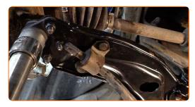
Screw in the fastening bolts of the bracket that connects the stabilizer bar to the front side of the control arm. Use a drive socket #13. Use a ratchet wrench.
