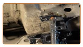
Connect the stabilizer bar to the control arm.
