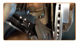
Install the fastening nut of the ball joint.
