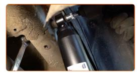
Tighten the top shock absorber fastening. Use a drive socket #18. Use a torque wrench. Tighten it to 50 Nm torque.
