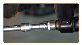
Screw the upper fastener of the shock absorber. Use a drive socket #18. Use a combination spanner #22.
