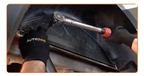
Tighten the lower fastener of the shock absorber. Use a drive socket #21. Use a combination spanner #21. Use a torque wrench. Tighten it to 110 Nm torque.
