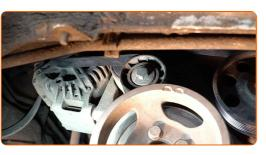
Install the hydraulic power steering belt. Turn the crankshaft pulley. Use a drive socket #E18. Use a ratchet wrench.
