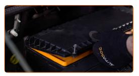
Screw in the fastening screws of the air filter cover. Use a drive socket #8. Use a ratchet wrench.
