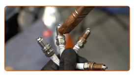
Install the new spark plugs into their mounting seats. Use the spark plug socket #16.
