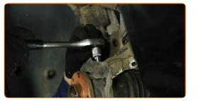
22 Release the fastener connecting the ball joint to the steering knuckle. Use a flat metal-working chisel. Use a hammer.
