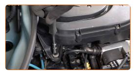
Remove the air filter housing retaining spring.
