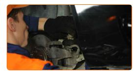
Connect the tie rod end to the steering knuckle and tighten it. Use a drive socket #17. Use a torque wrench. Tighten it to 40 Nm torque.
