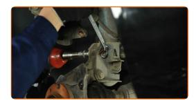
Unscrew the ball joint fastening to the steering knuckle. Use a combination spanner #13. Use a drive socket #13. Use a ratchet wrench.
