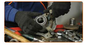
Install the retaining ring in the steering knuckle. Use a flat screwdriver.
