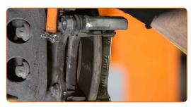
Unscrew the caliper bracket fastening. Use a combination spanner #13.
