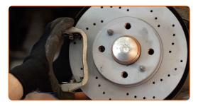
Tighten the brake caliper bracket. Use a combination spanner #13. Use a torque wrench. Tighten it to 54 Nm torque.
