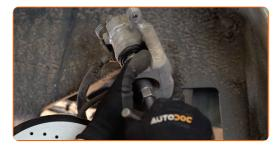
Install the brake caliper and fix it. Use a combination spanner #17. Use a drive socket #13. Use a ratchet wrench. Use a torque wrench. Tighten it to 27 Nm torque.
