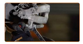
g Remove the brake caliper.
