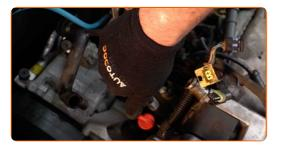
Screw new spark plugs and tighten them. Use the spark plug socket #16. Use a torque wrench. Tighten it to 27 nm torque.
