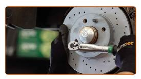
20 Install the brake caliper bracket.
