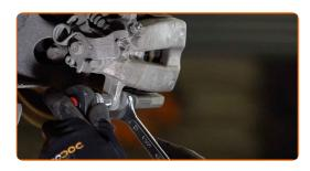
g Remove the brake caliper.
