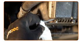
Screw in the new drainage plug and tighten it. Use a drive socket #17. Use a torque wrench. Tighten it to 22 Nm torque.
