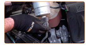
Attach the fuel pressure sensor connector.
