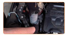
Detach the fuel pressure sensor connector.
