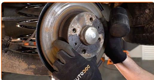
**17** Clean the hub. Use a wire brush. Treat the contacting surface. Use copper grease.
