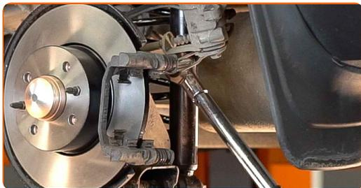
**23** Treat the brake caliper piston. Use a brake cleaner.
