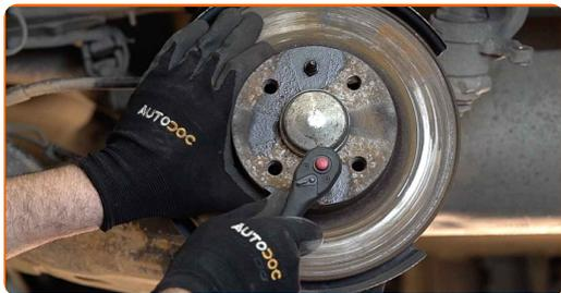
**16** Remove the brake disc. Use a rubber mallet.
