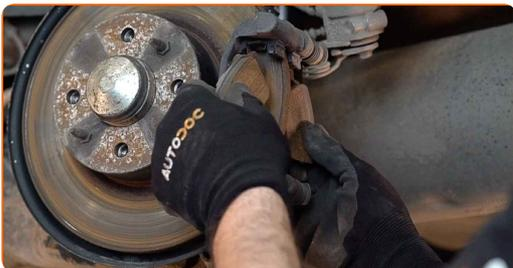
**11** Clean the brake caliper bracket fasteners. Use a wire brush. Use WD-40 spray.
