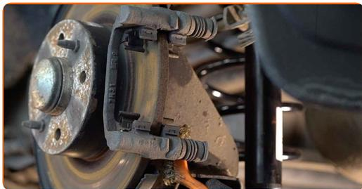
**12** Unscrew the caliper bracket fastening. Use a drive socket #17. Use a tap wrench.
