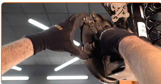
**22** Tighten the brake caliper bracket. Use a drive socket #17. Use a torque wrench. Tighten it to 62 Nm torque.
