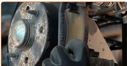
**14** Clean the brake disc fasteners. Use a wire brush. Use WD-40 spray.
