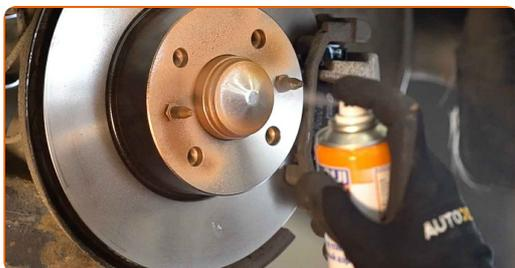
**29** Clean the brake disk surface. Use a brake cleaner.
