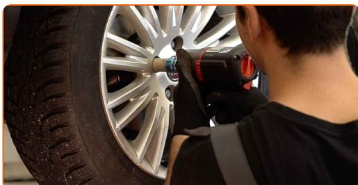
**32** Lower the car and working in a cross order, tighten the wheel bolts. Use a torque wrench. Tighten it to 120 Nm torque.
