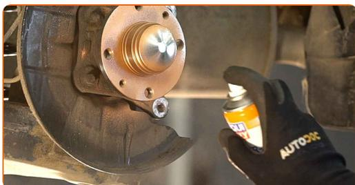
**18** Install the brake disc.
