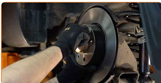
**19** Tighten the brake disc fastening. Use a drive socket #12. Use a torque wrench. Tighten it to 10 Nm torque.
