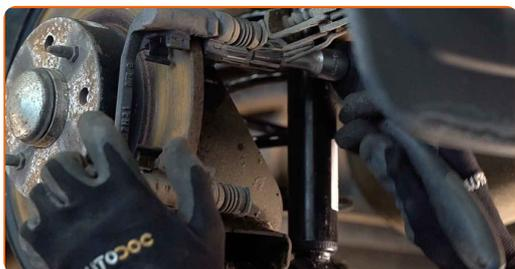
**13** Remove the caliper bracket.
