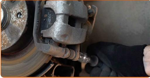
**9** Remove the brake caliper. Use a crowbar.
