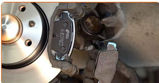
**26** Install the brake caliper and fix it. Use a drive socket #13. Use a torque wrench. Tighten it to 30 Nm torque.
