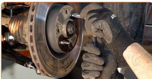
18 Remove the brake disc.
