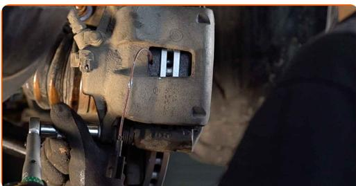
**29** Connect the brake pad wear sensor plug.
