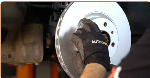
21 Tighten the brake disc fastening. Use a drive socket #12. Use a torque wrench. Tighten it to 10 Nm torque.
