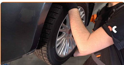
**7** Disconnect the brake pad wear sensor plug.
