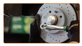
20 Install the brake caliper bracket.
