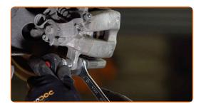
g Remove the brake caliper.
