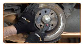
Remove the brake disc. Use a rubber mallet.
