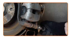
Remove the brake caliper. Use a crowbar.
