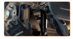
Remove the caliper bracket.
