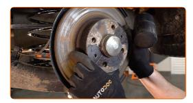
Remove the hub bearing protection cap. Use a crowbar. Use a hammer.
