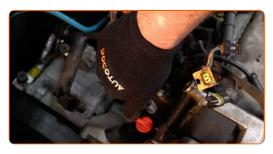
Screw new spark plugs and tighten them. Use the spark plug socket #16. Use a torque wrench. Tighten it to 27 nm torque.
