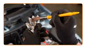
Install the new spark plugs into their mounting seats. Use the spark plug socket #16.
