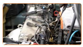
Unscrew the spark plugs. Use the spark plug socket #16. Use a ratchet wrench.
