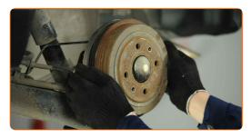
Remove the hub bearing protection cap. Use a flat screwdriver. Use a hammer.
