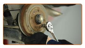
10 Remove the brake drum.
