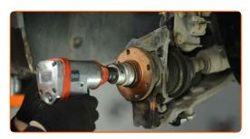
Restake the wheel hub retaining nut. Use a pin punch. Use a hammer.
