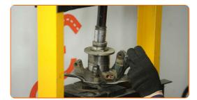
Tighten the lower fasteners connecting the shock strut to the steering knuckle. Use a combination spanner #17. Use a drive socket #17. Use a torque wrench. Tighten it to 75 Nm torque.
