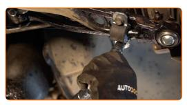
Treat all joints of the stabiliser link. Use copper grease.
